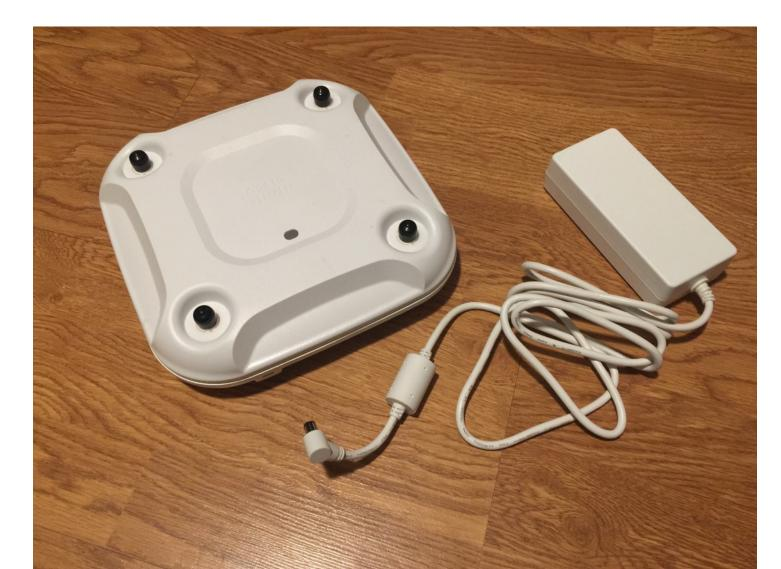
This is the AC/DC supply that can be purchased with the Access Point, used to power the AP from an AC outlet.
