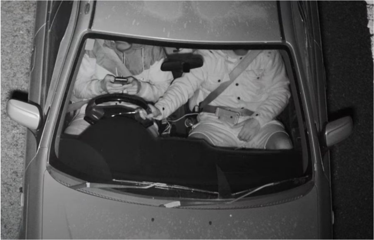
Example of Thermal Flash (gray scale infrared) photo from Distracted Driving Detection Camera
