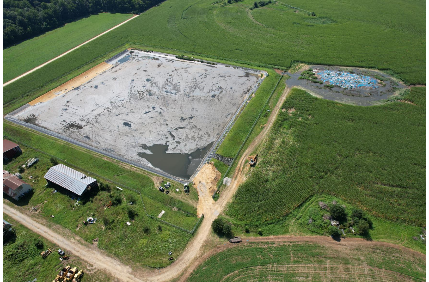
Image 7: Aerial of drained and lagoon and sludge from the lagoon stored on the ground uncontrolled (8-18-2023)
