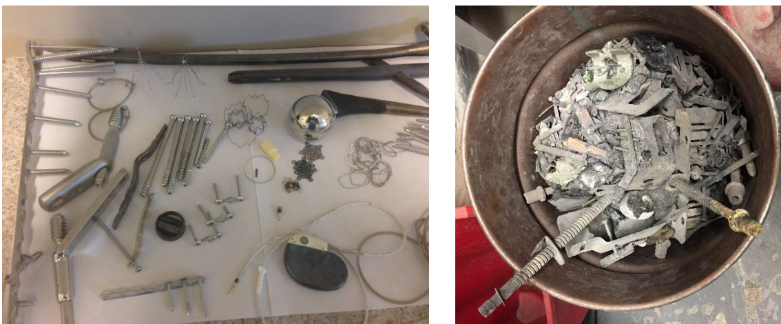
Above: Medical implants recovered from Aquamation on the left, and medical implants recovered from flame cremation on the right. Notice that with Aquamation, the implants are in excellent condition, and that pacemakers do not have to be removed.
