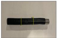
◆ This image shows the "black" arc-resistive, single-layer jacket CSST. This product meets requirements from 2022's HB 1052. You can see a perforation from a lightning-induced arcing event, which caused a fire to a single -family home in Ellicott City in 2021.
