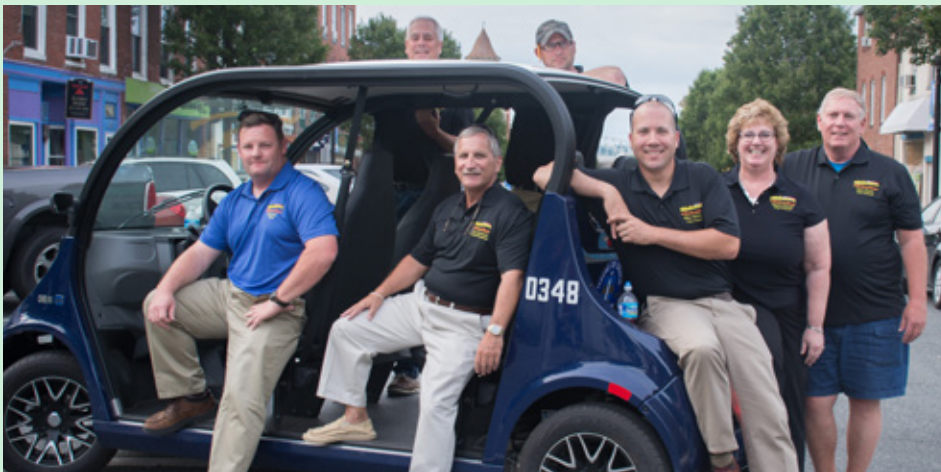
Havre de Grace purchased two Polaris/GEM cars to replace standard six-cylinder automobiles for short trips around the City. The operating cost of 3 cents per mile for the GEM cars compared with 12 to 14 cents per mile for standard autos saves money and reduces the carbon footprint.
