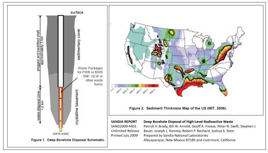
Left: Deep Borehole Disposal Schematic. Right: Depth the Crystalline Basement Map
