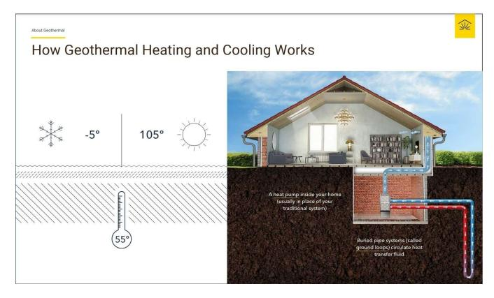
Geothermal heat pumps work by collecting heat from the ground, where it remains a constant 55 degrees Fahrenheit year-round and transferring it to heat a home or business. In the summer, the system works in reverse, collecting heat from the building and transferring it to the ground.
