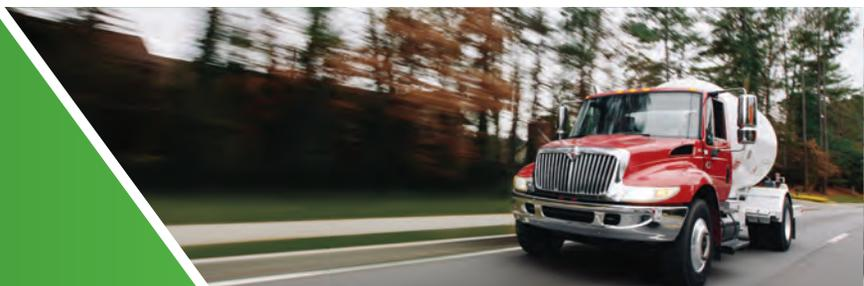
Tanks used in smaller bobtail delivery trucks and larger highway transport vehicles have capacities that range **from 3,000 – 12,000 gallons** and are built of thick, high-strength steel.
