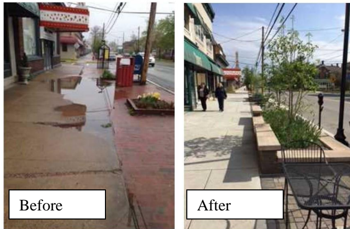
Figure 1: Impact of street tree planter boxes on flooding. Prior to this Chesapeake Bay Trust-funded urban greening grant, local business basements flooded. After the project, businesses report no basement flooding.
