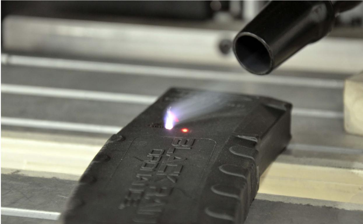
Here you can see a magazine catching fire using the settings from a known German polymer on this unknown polymer. The result is:
