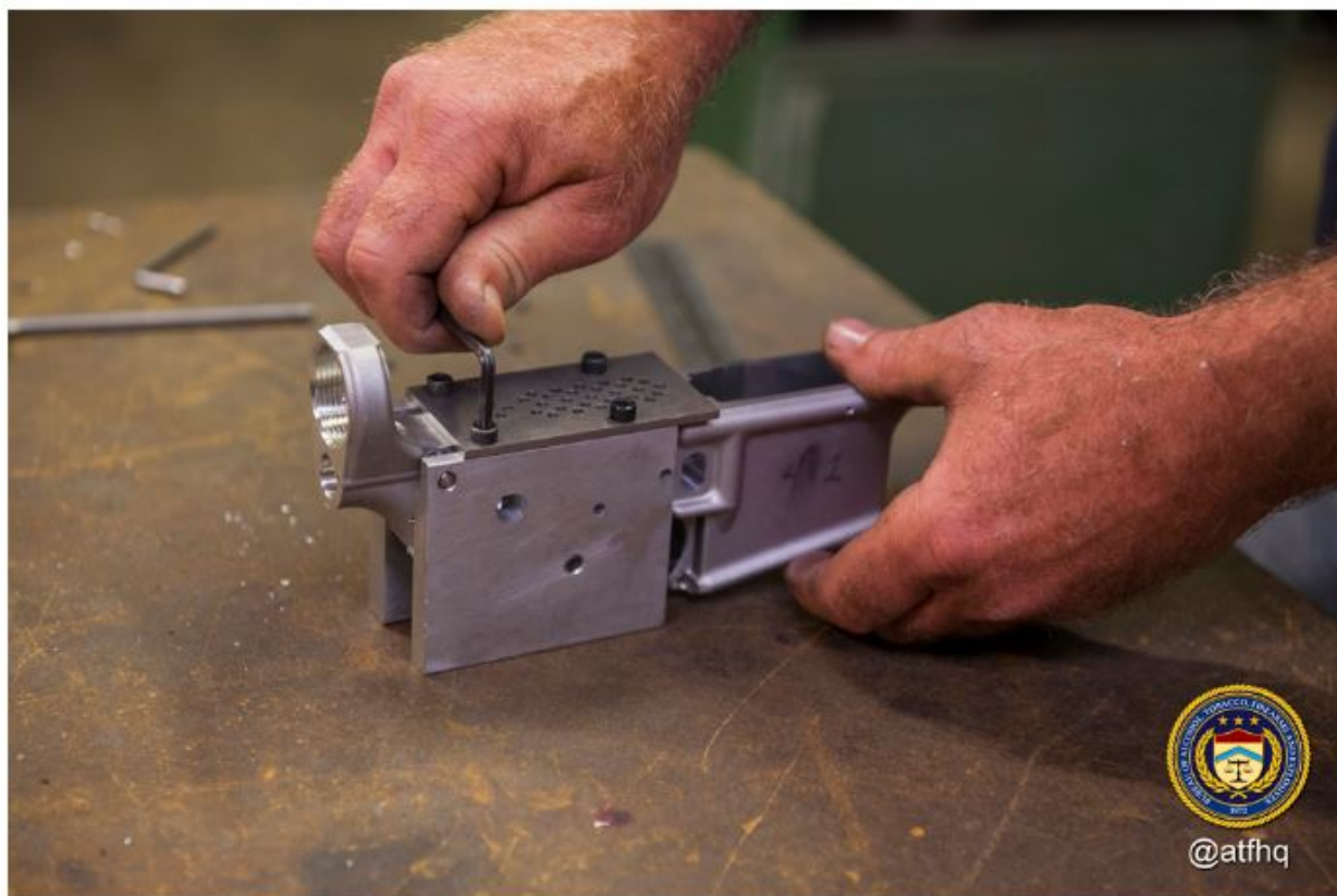
Attaching first drilling template for fire control cavity
