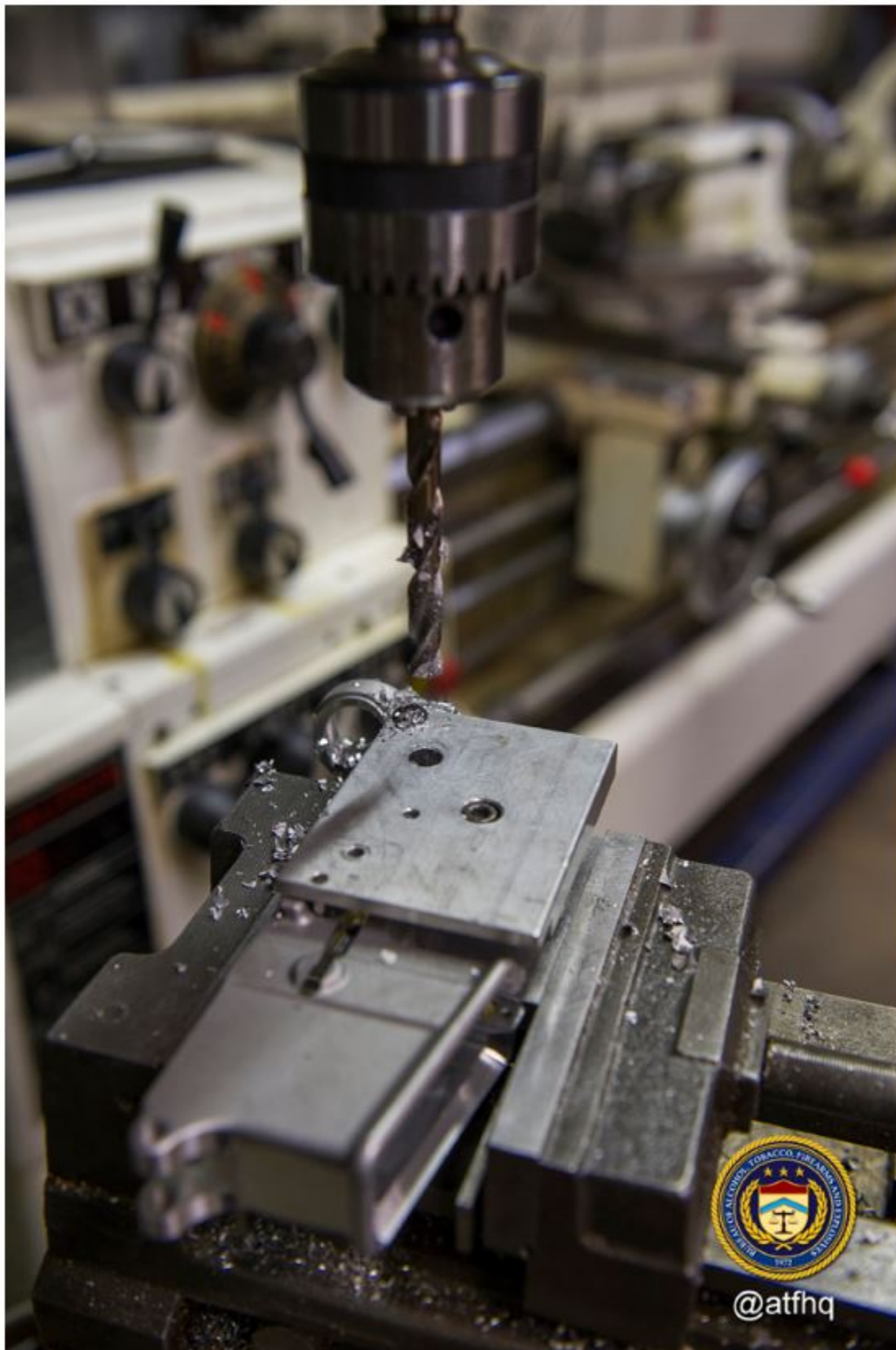
Setup for drilling selector hole
