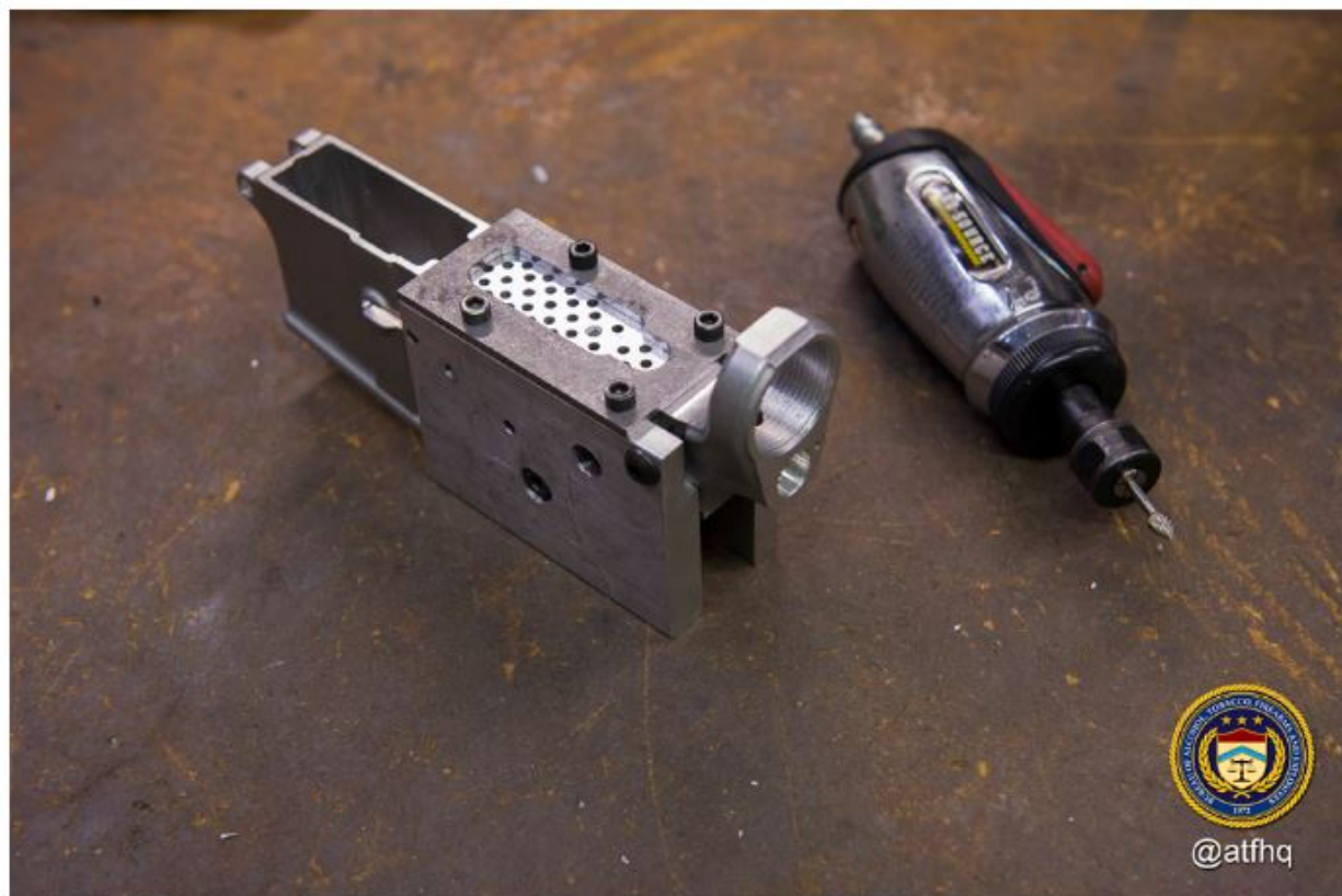
Attached milling template for fire control cavity
