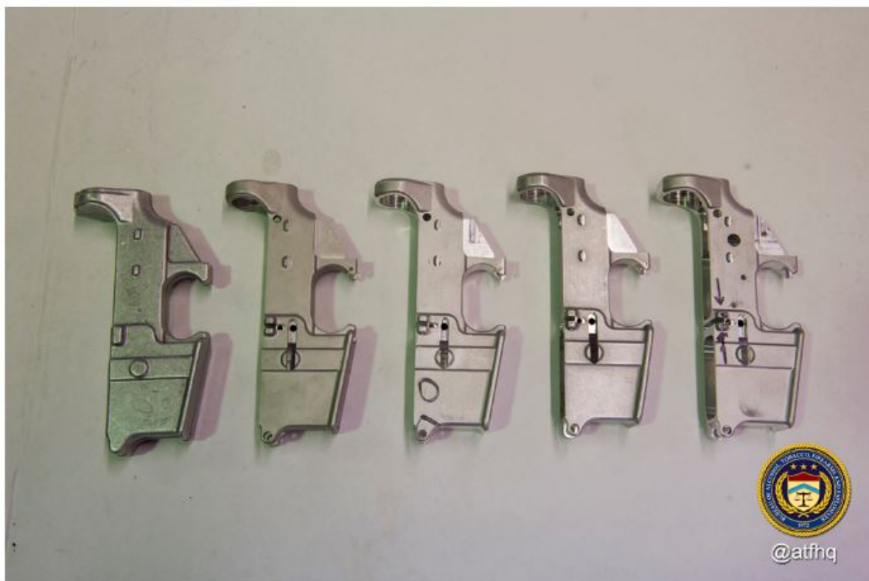
Various stages of completion (side view)
