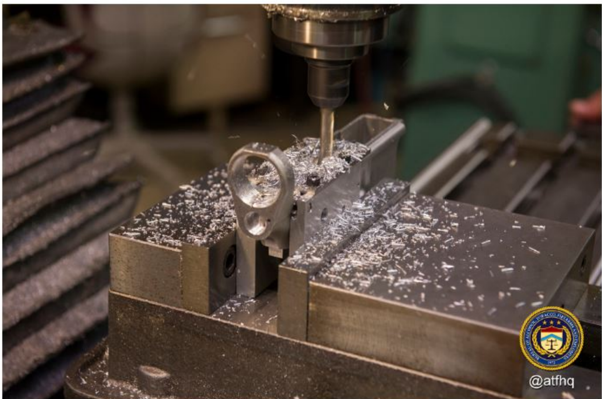
Milling material from fire control cavity
