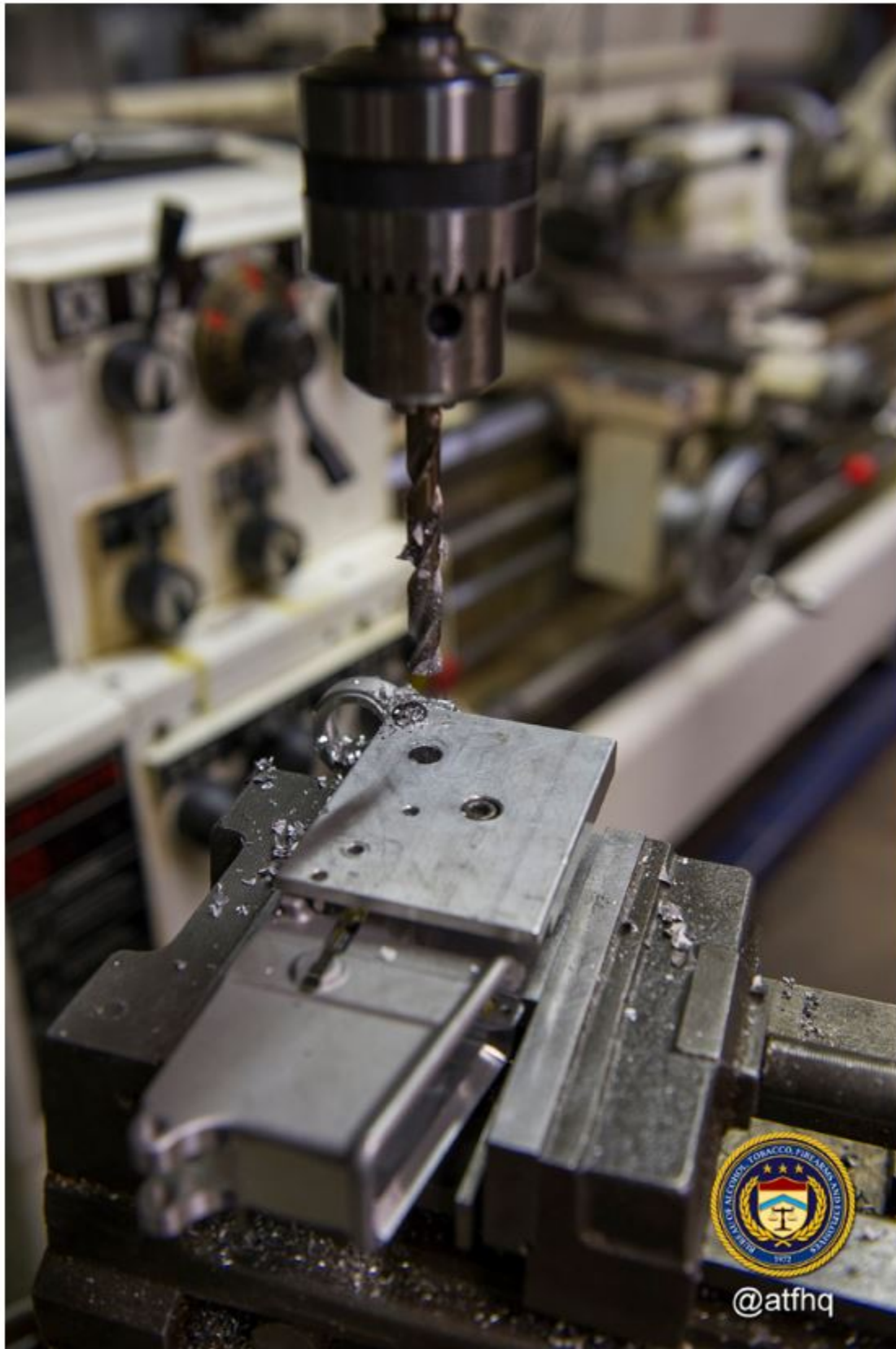
Setup for drilling selector hole
