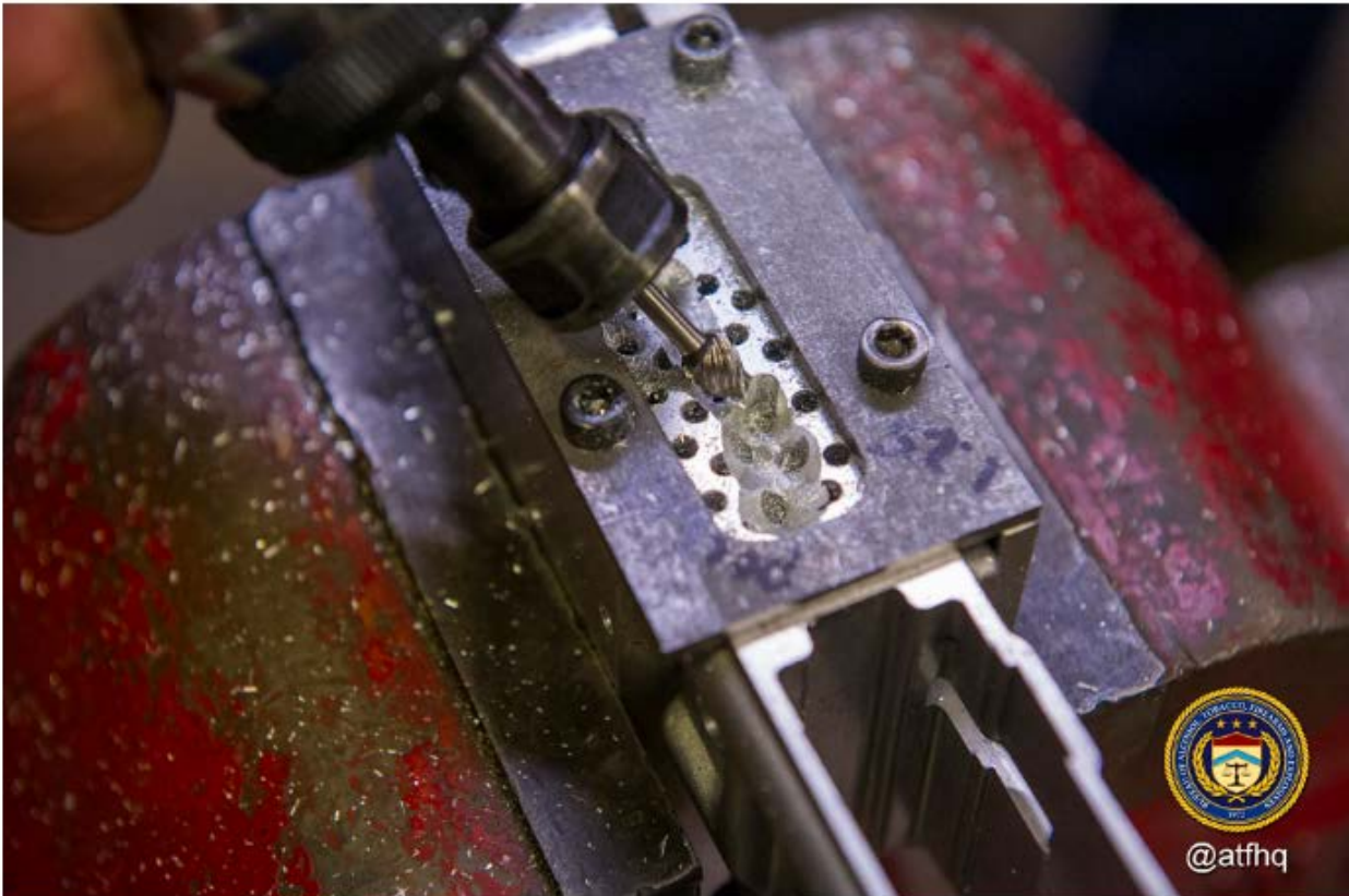
Removing material from fire control cavity with rotary tool
