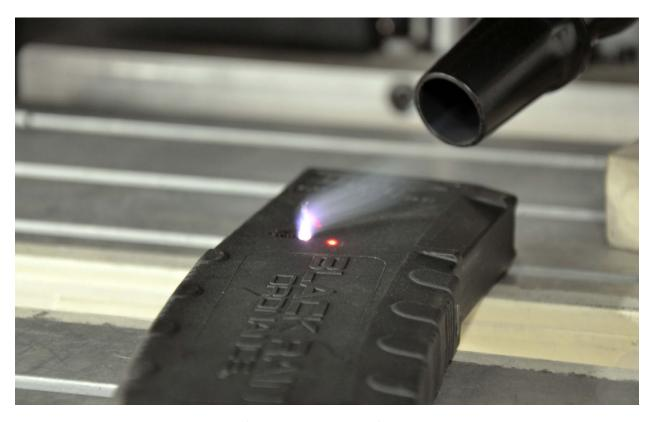
Here you can see a magazine catching fire using the settings from a known German polymer on this unknown polymer. The result is:
