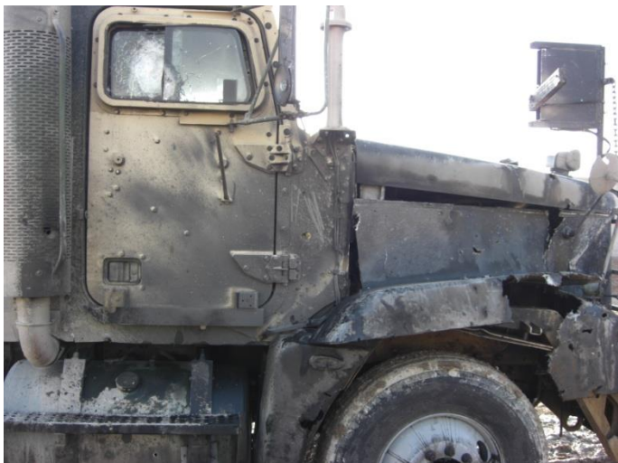
Figure 1: The passenger side of the M915 truck showing the damage caused by the IED.
