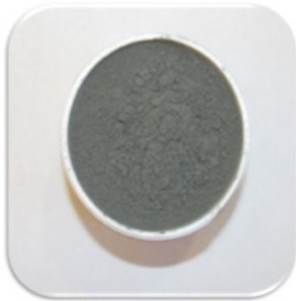
Untreated Fly Ash 12% LOI 250 ppb Mercury
