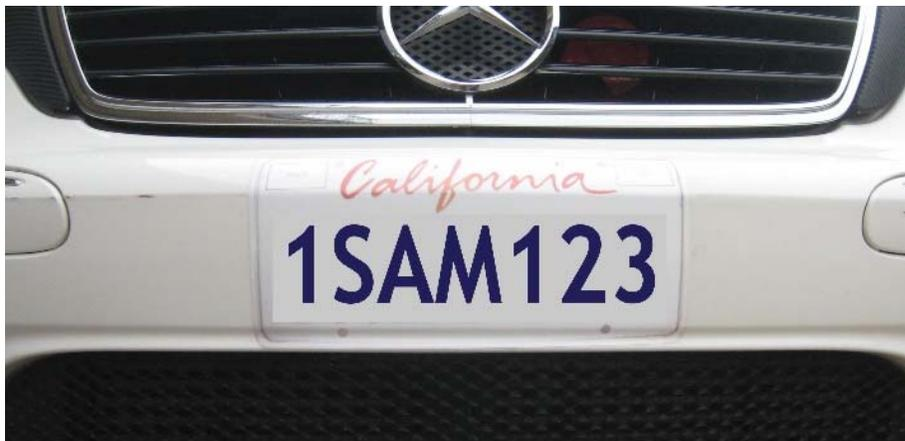
During the pilot, the vendor used three different wrapping materials. From testing, the CHP reported that the standard California white version of the License Plate Wrap in all three materials were visible and readable by the human eye observer and detectable by the ALPR at various light conditions, distances, angles, and satisfied statutory requirements related to plate size and reflectivity.
