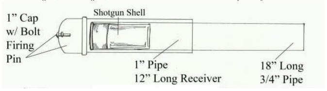
The zip gun in the diagram functions by inserting the shotgun shell into the "barrel" piece, then sliding the "receiver" piece over the end. Sliding the two pieces together forces the firing pin in the pipe cap into contact with the primer in the shotgun shell, initiating the explosive process.
