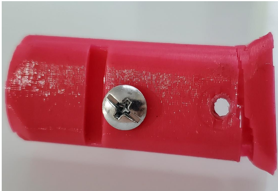
Figure 1 - Layer Line fracture
