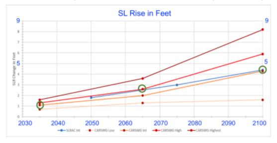
**Exhibit 4.** The recommended new seawall is 5.2 feet above current MSL Future MSL and 100 year flood levels based on rising MSL are shown at three dates.
