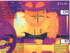
Low Pressure Steam Valve Operating Temperature, \*F Ambient Temperature, \*F Insulation selected
