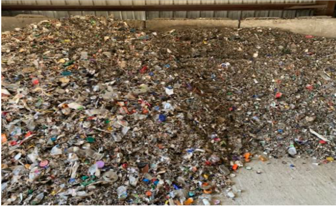
Picture of a Commingled Single Stream Recycled “Glass” - as delivered from a Materials Recovery Facility. Requires intensive sorting and cleaning prior to meeting furnace-ready specifications.
