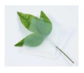
A clear wood material that is lighter and tougher than glass, with up to 3x better thermal insulation. It also offers benefits in terms of both light channeling (to reduce glare) and far more environmental sustainable.
