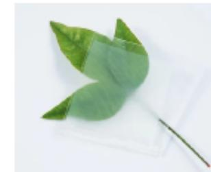
A clear wood material that is lighter and tougher than glass, with up to 3x better thermal insulation. It also offers benefits in terms of both light channeling (to reduce glare) and far more environmental sustainable.
