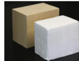
A bright-white material that is stronger than natural wood and insulates against both heat loss and impacts better than commercially available alternatives. It is also biodegradable and eco-friendly.
