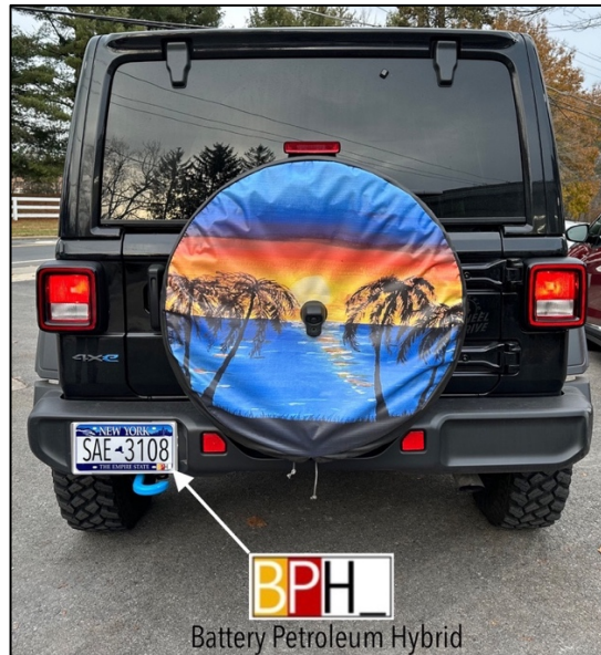
Figure 5. SAE J3108 license plate marking (sticker) for firefighter awareness about alternative fuels and power sources.
