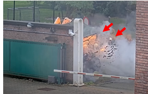
Figure 4. Jeep exploding after firefighters broke a window to ventilate the interior. Arrows point to firefighters caught in blast.
