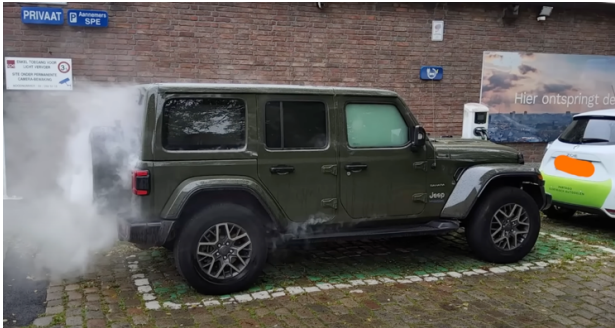
Figure 3. Jeep plug-in hybrid undergoing battery failure was hard to differentiate from non-hybrid Wranglers. The cabin was full of flammable vapors. (Belgium 10/30/23)
