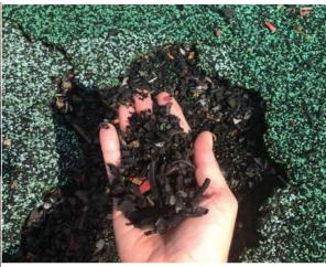
As unitary synthetic surfacing begins to age, it may deteriorate and expose the loose-fill cushioning layer underneath. This layer is typically made with shredded waste tires.
