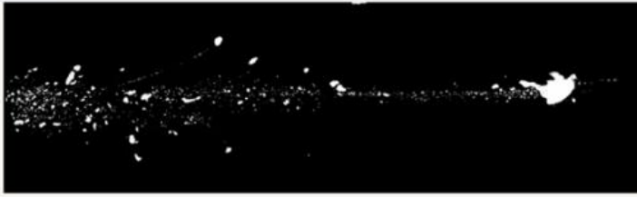
Traditional lead bullet fragmentation on entry
