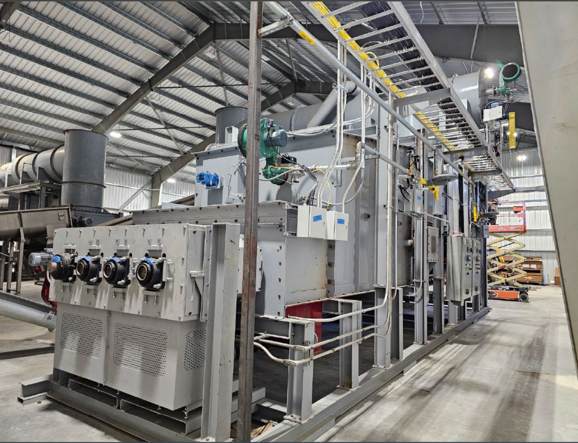
Earthcare's sewage sludge gasifier in Berks County, PA
