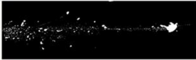
Traditional lead bullet fragmentation on entry
