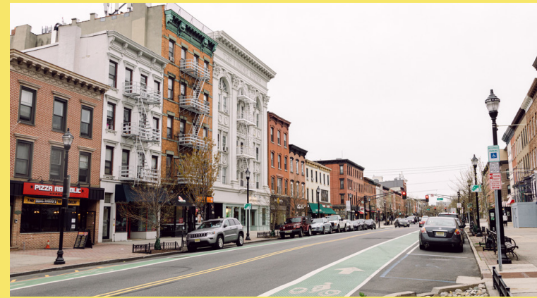
Top: Streetscape of Adams Street in Hoboken, New Jersey, featuring a bumpout curb extension greenscape. Curb extensions are part of the "daylighting" strategy to increase visibility. Photo by Shutterstock
