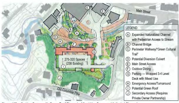
Figure 167: Parking Garage with Green Roof Elements, Mixed Use Space and Activated Channel
