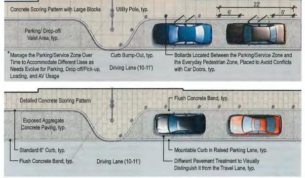
Figure 105: Potential Streetscape Improvements and Pavement Scoring Options. The raised parking/drop-off area with mountable curb concept will likely only be possible along Maryland Avenue and lower Main Street where curb lines can be potentially shifted with the removal of the four buildings as part of EC Safe and Sound.
