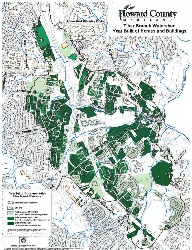
Figure 36: Development Year and Stormwater Management Required, Darkest Green Identifies Properties that were Developed Prior to 1984 with No Required Stormwater Management, Credit: Howard County DPZ
