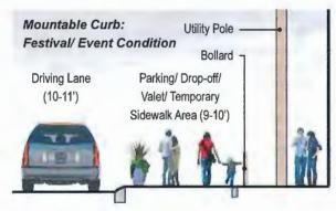
Figure 102: Flexible Use Zone with Mountable Curb Concept Section, For Illustrative Purposes Only, The raised parking/drop-off area with mountable curb concept will likely only be possible along Maryland Avenue and lower Main Street where curb lines can be potentially shifted with the removal of the four buildings as part of EC Safe and Sound.
