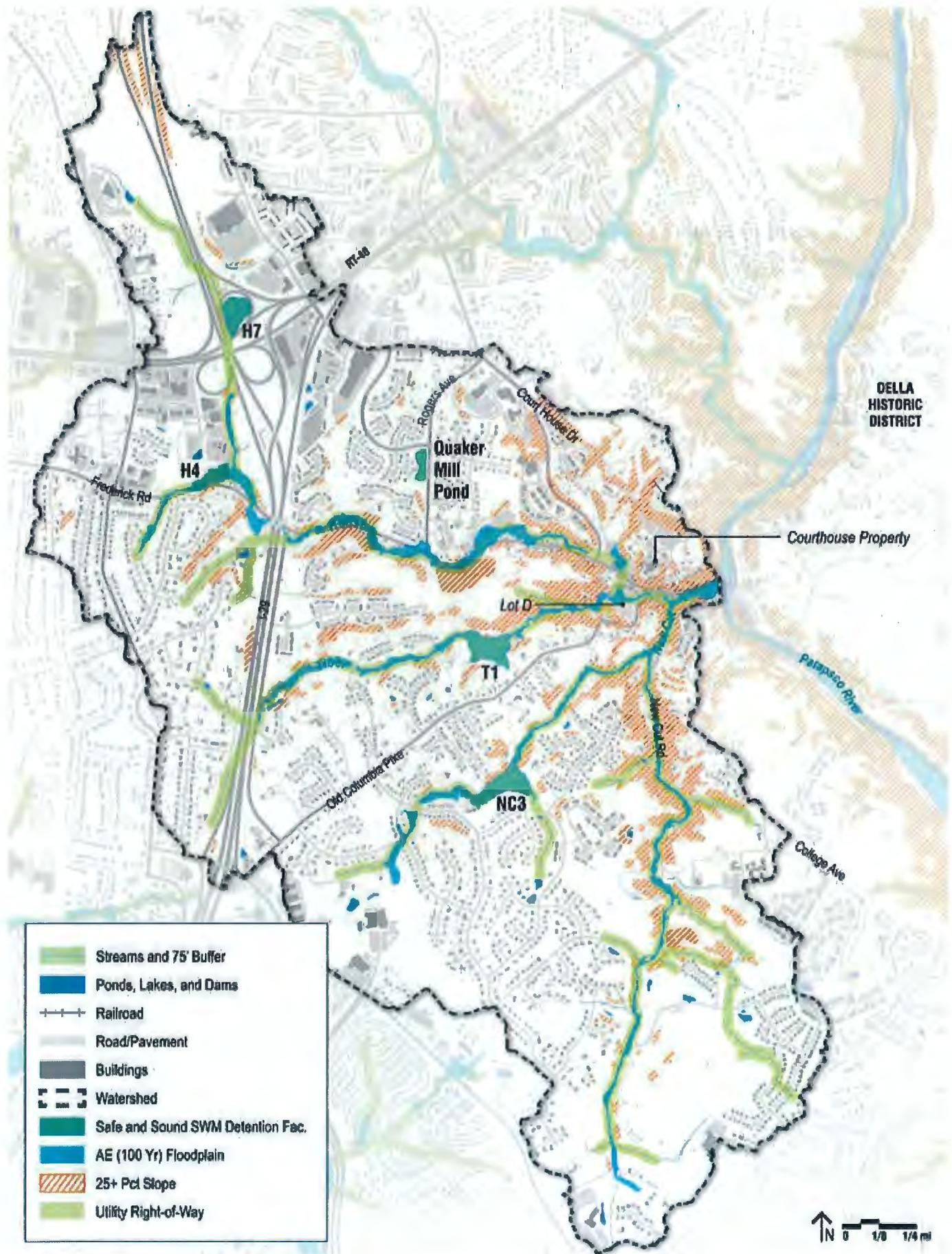
Figure 35: Watershed Diagram: Hydrology and Steep Slopes
