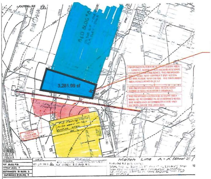
Make sure the fence foundation is not overlapping with 6" TAP and RCP
